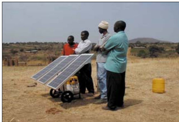
Harvester with water purification package
